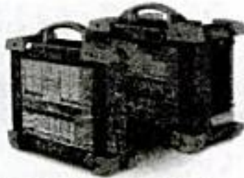
Fig. 14.20 Example of portable universal test sets that can be used for OTDR traces, optical spectrum analysis, dispersion analysis, and other test functions. (Model FTB-400, photo provided courtesy of EXFO; www.exfo.com.)
